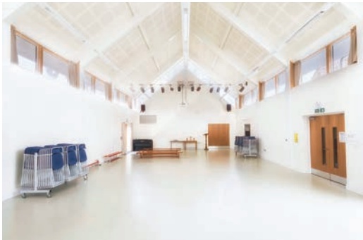
High level glazing providing good lighting and ventilation in the hall
